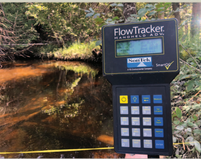
A FlowTracker calculates the amount and speed of water flowing in the Little Pigeon River.
