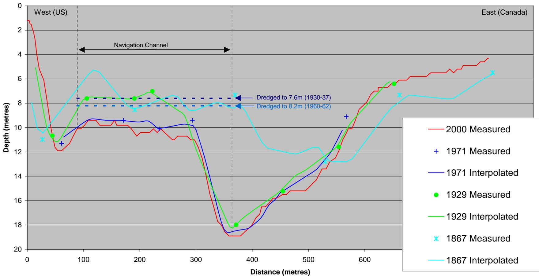
Figure 3.6 Profile A Bathymetry Comparison 1867, 1929, 1971 and 2000
