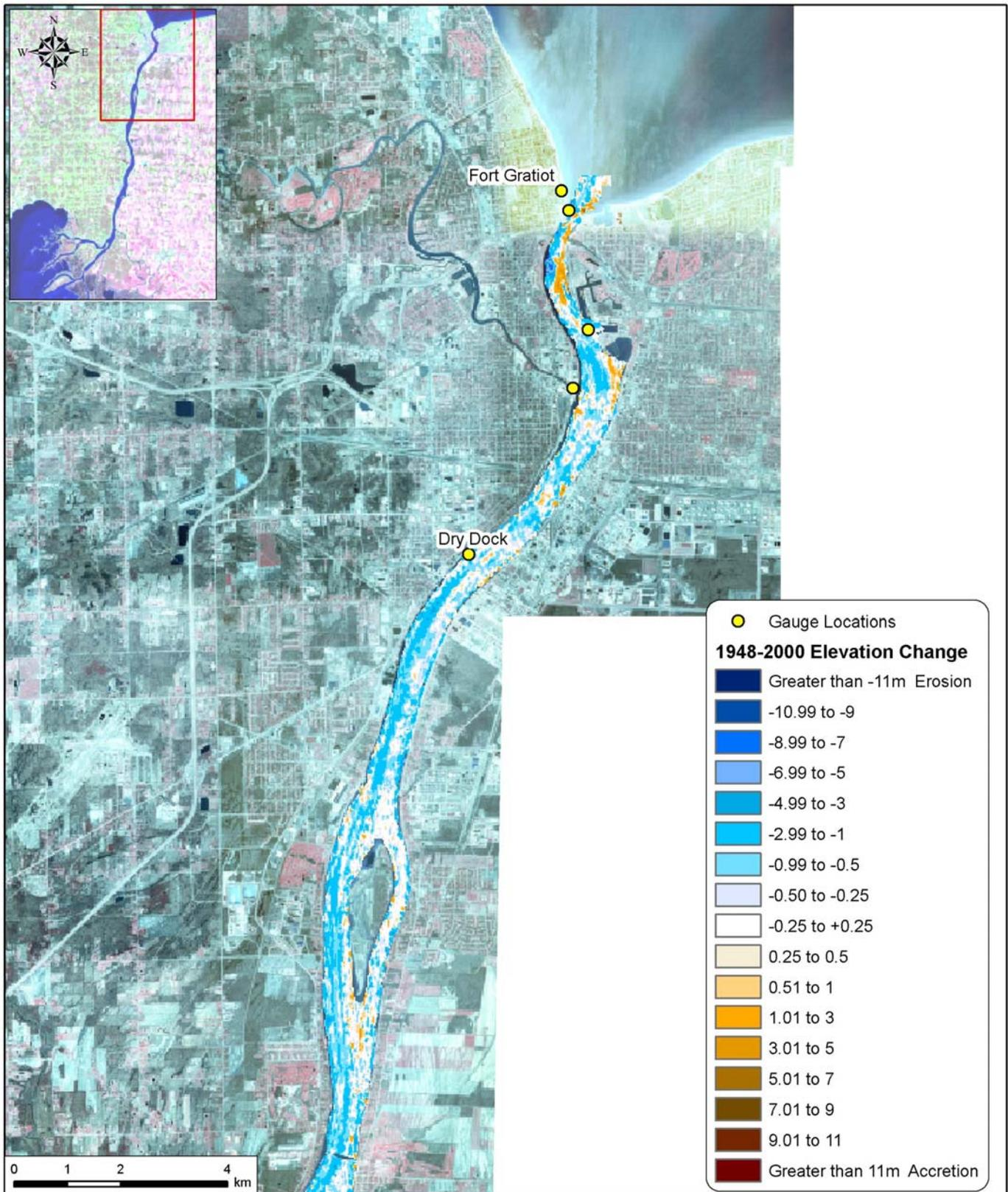
Figure 4.6a Bathymetry Change 1948 to 2000 (North Reach St. Clair River)
