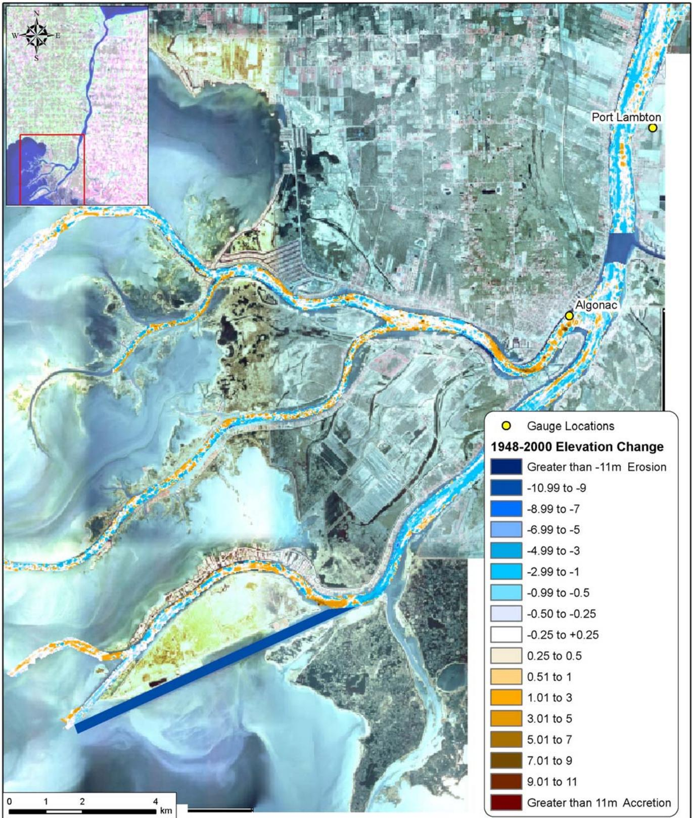
Figure 4.6c Bathymetry Change 1948 to 2000 (Delta St. Clair River)
