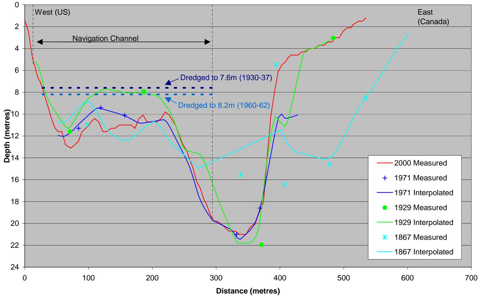
Figure 3.7 Profile B Bathymetry Comparison 1867, 1929, 1971 and 2000
