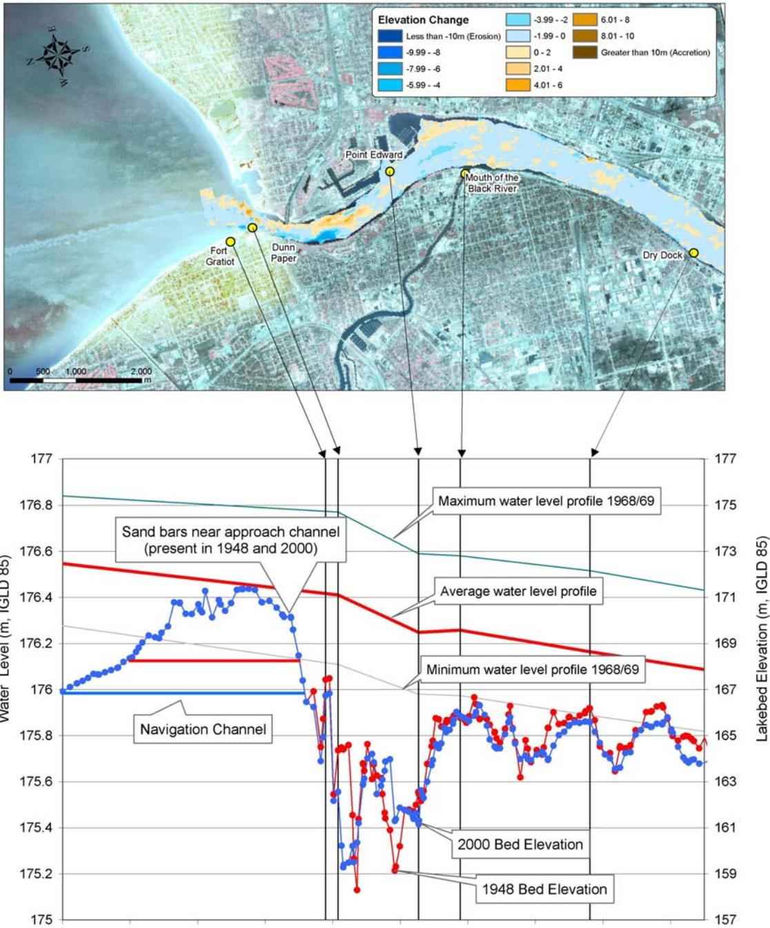
**Figure F River Bed Change (1948-2000) and Water Surface Profiles in the St. Clair River**
