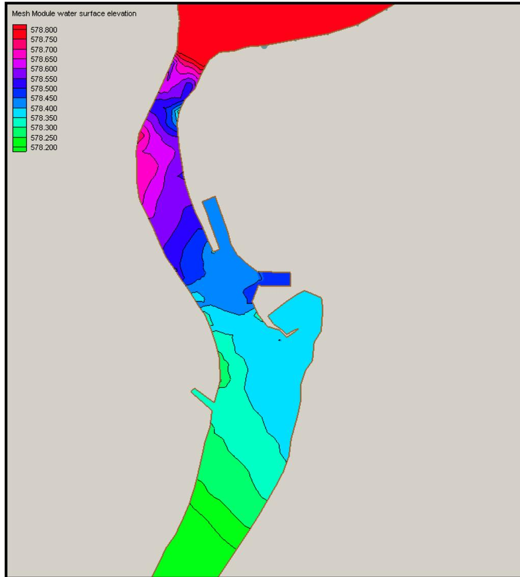
**Figure 5.3 Water Surface Elevation from RMA2 Validation Run**
