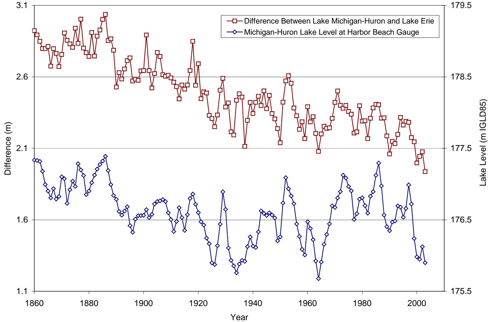
Figure C Comparison of Level Difference (MH-E) and MH Lake Levels
