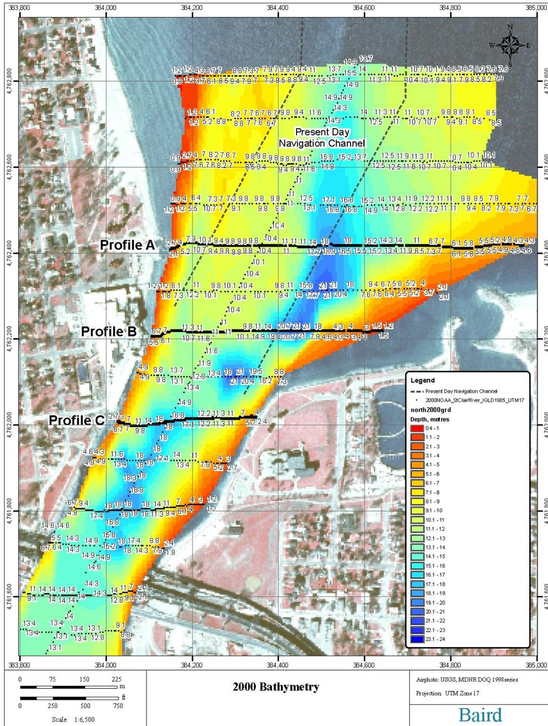
**Figure 3.4 Bathymetry at St. Clair River Inlet in 2000**
