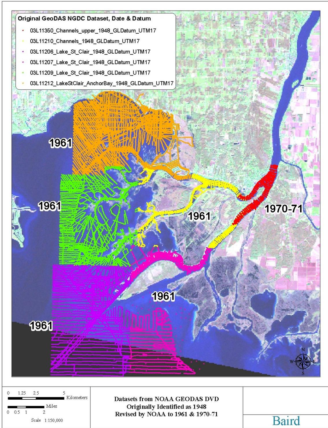
**Figure A3 Bathymetry Data from NOAA GEODAS DVD Revised from 1948 to 1961, 1970-71**
