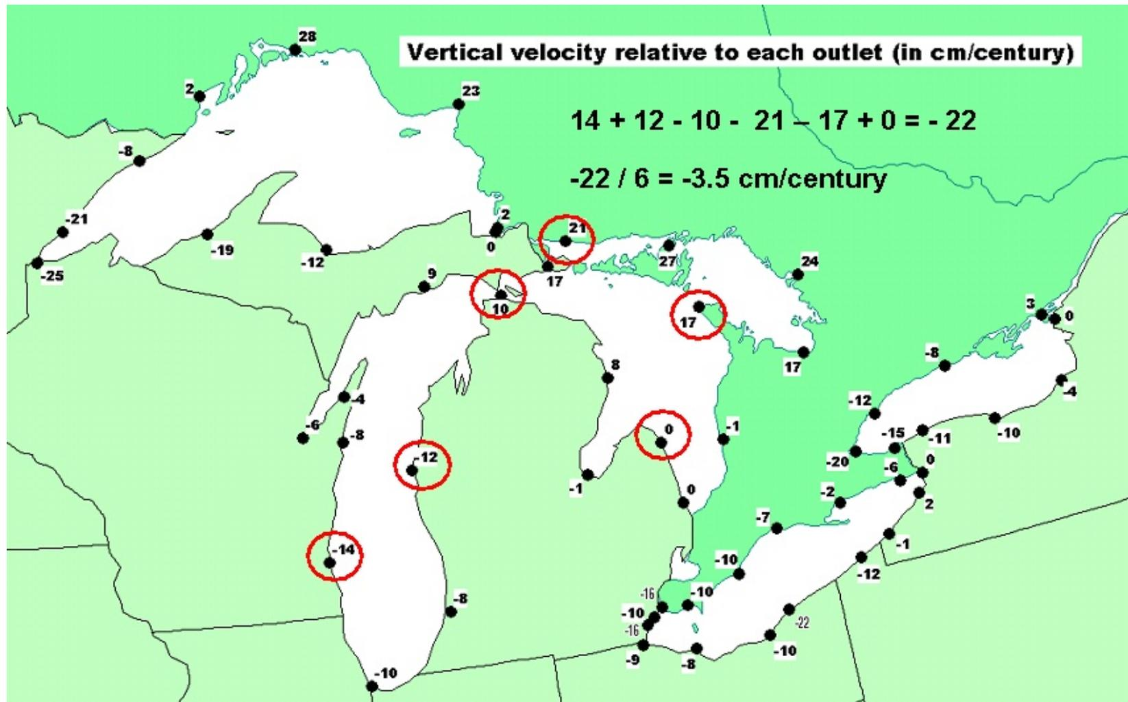
Figure 3.4 Relative Crustal Movement with Respect to Lakewide Average at the Water Level Gauge Network (provided by C. Southam, Env. Canada)
