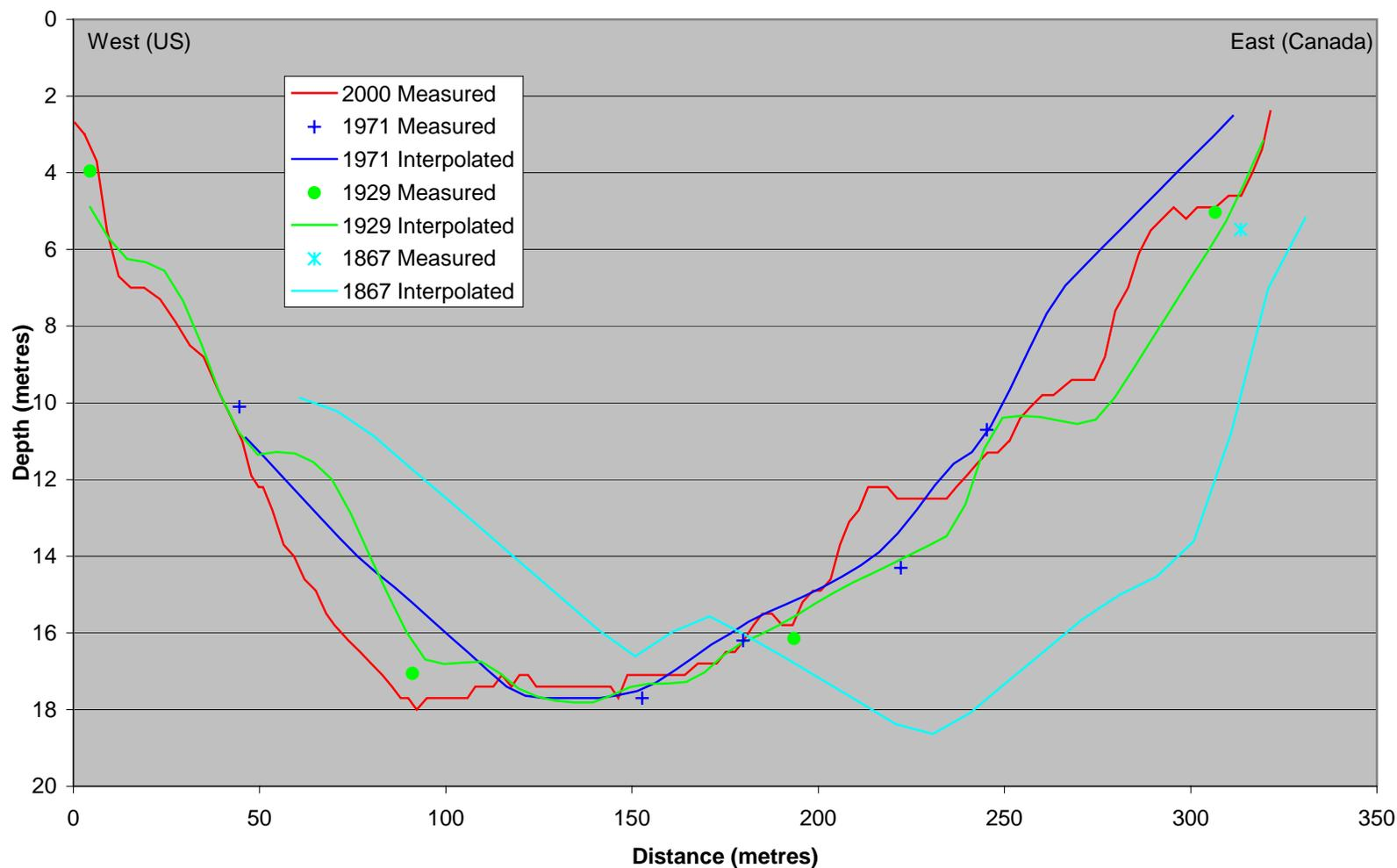
Figure 3.8 Profile C Bathymetry Comparison 1867, 1929, 1971 and 2000
