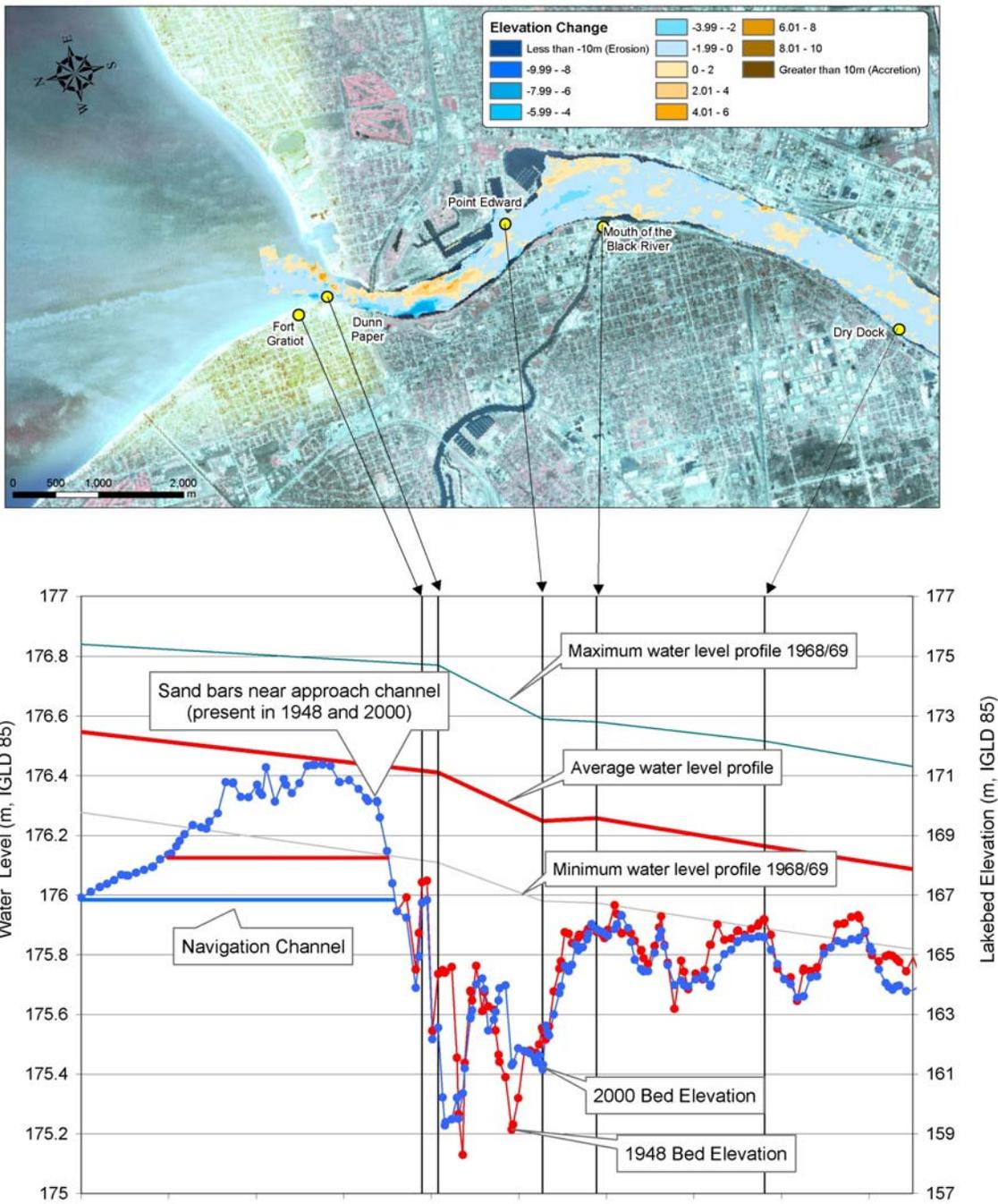
**Figure 5.8 River Bed Change (1948-2000) and Water Surface Profiles in the Upstream End of the St. Clair River**
