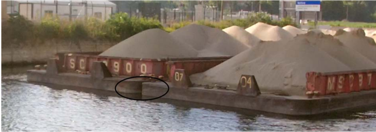
Figure 4. Picture of the front of a rake-to-rake barge configuration traversing the electrical barrier with the square ends in the front. The circle denotes the small void space that two live fish swam into and remained inside beyond the barrier.
