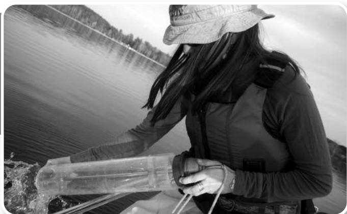
Restoration Ecologist, Jennifer Gelb, uses a Kemmerer bottle to collect water samples.
