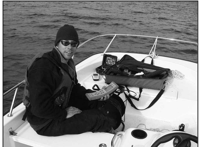
Kevin Cronk, our Monitoring and Research Coordinator, uses the Hydrolab™ to measure water quality.
