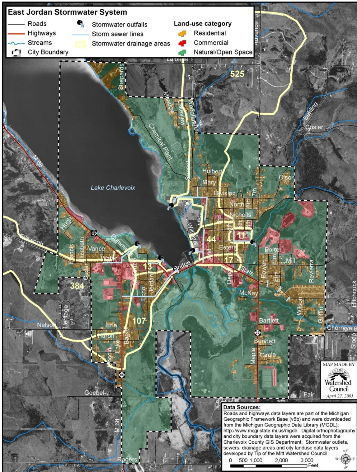
Figure 24: City of East Jordan stormwater system
