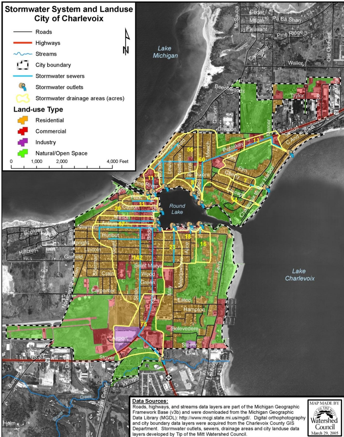
Figure 23: City of Charlevoix stormwater system
