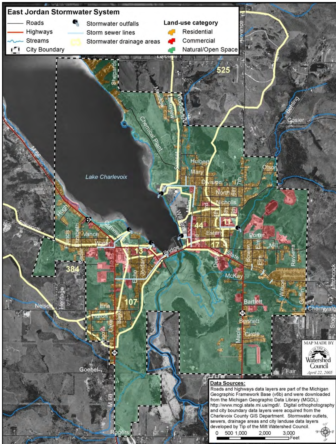
Figure 24: City of East Jordan stormwater system
