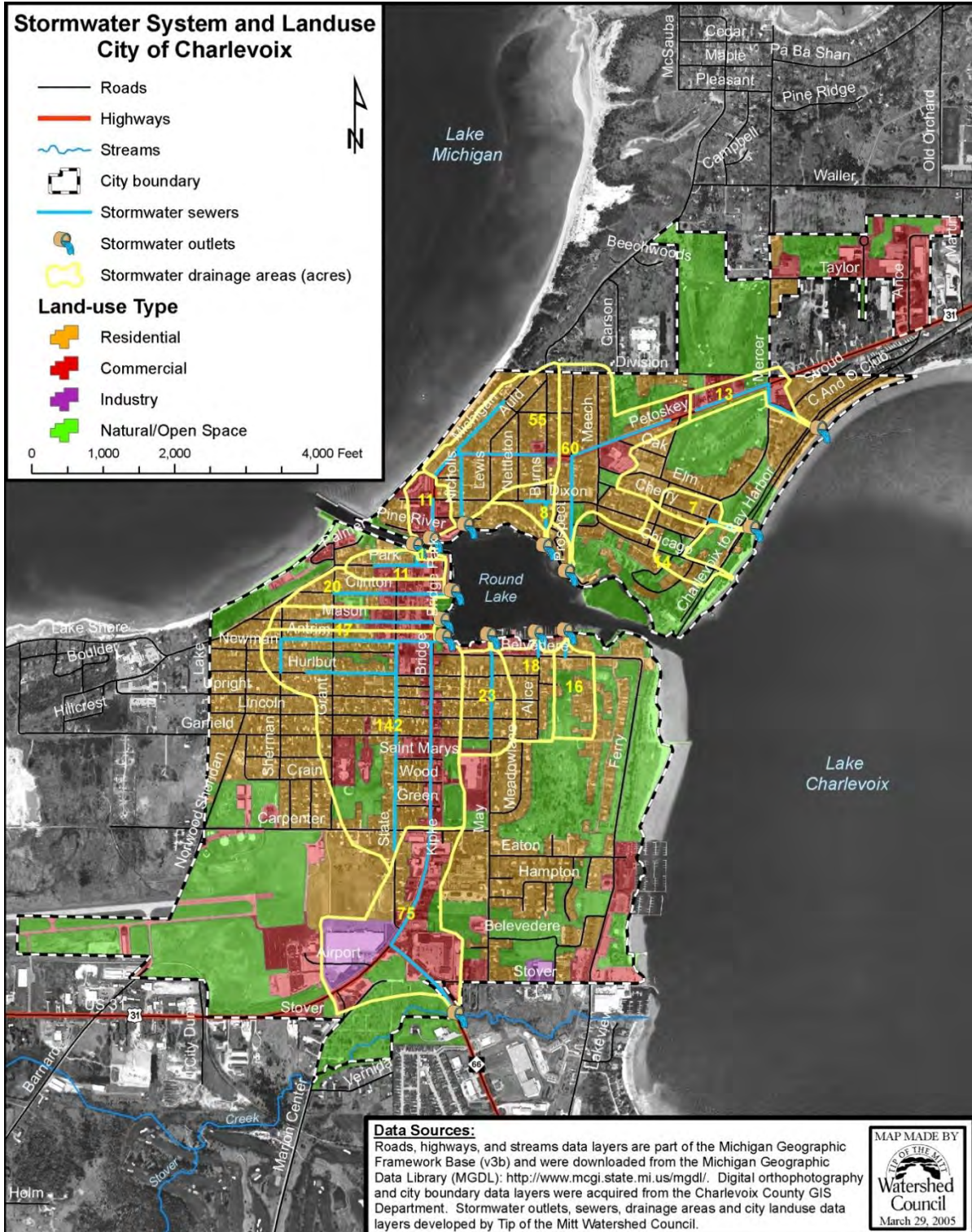
Figure 23: City of Charlevoix stormwater system
