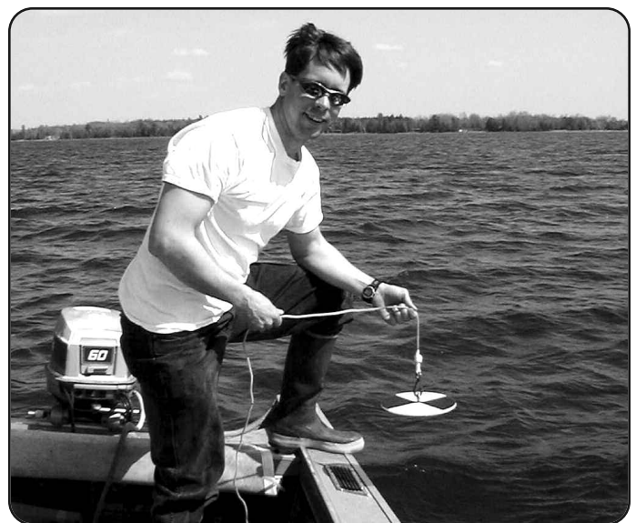
Kevin Cronk, our Monitoring and Research Coordinator, measures the water clarity on Paradise Lake with a secchi disc. This is just one of the many tests done to thoroughly check the health of the lake.
