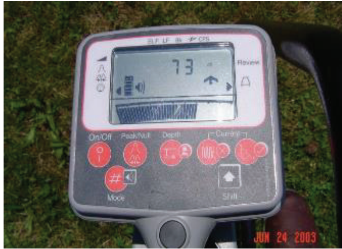
Figure 24: Picture of A Display from An ACVG Receiver
