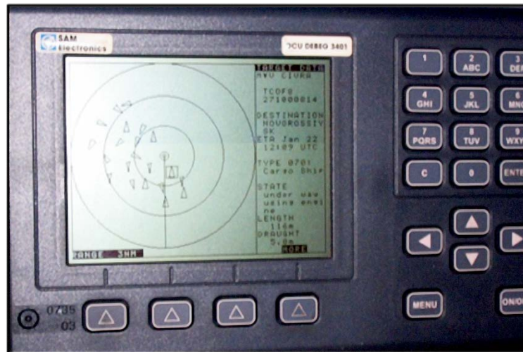
Figure 8: An AIS monitor mounted on a vessel.
